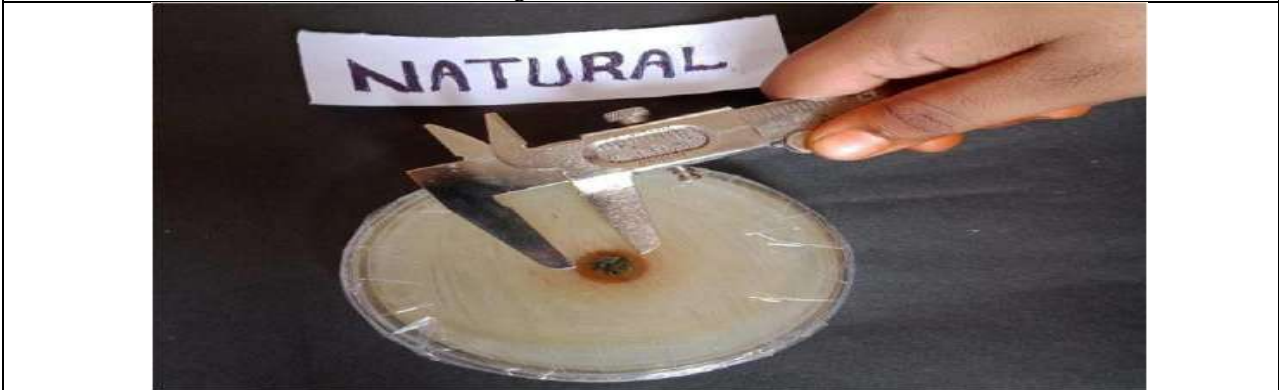
Fig 5. Measuring the zone of inhibition by using Vernier caliper
